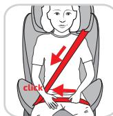
Make sure that the diagonal belt runs exactly and does not run too close to the child's neck. All straps must fit tightly against the child and must not be twisted.
