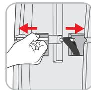
Afterwards you can loosen the harness belts (**G2**) and the shoulder pad belts (**SG**) from the adjustment unit and pull out both belt ends through the shoulder belt lead-through (**G1**).
