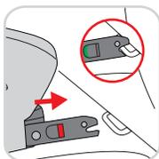
Now release the ISOFIX adjustment button (IE) and make sure that both clips do not slip back.
