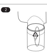
Rotate the trap door to the **OPEN** position.
