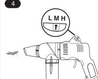
Place the nozzle next to the bug and activate the vacuum by pressing the trigger.
