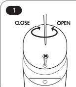
Open or close the cover with a cross-head screwdriver.
